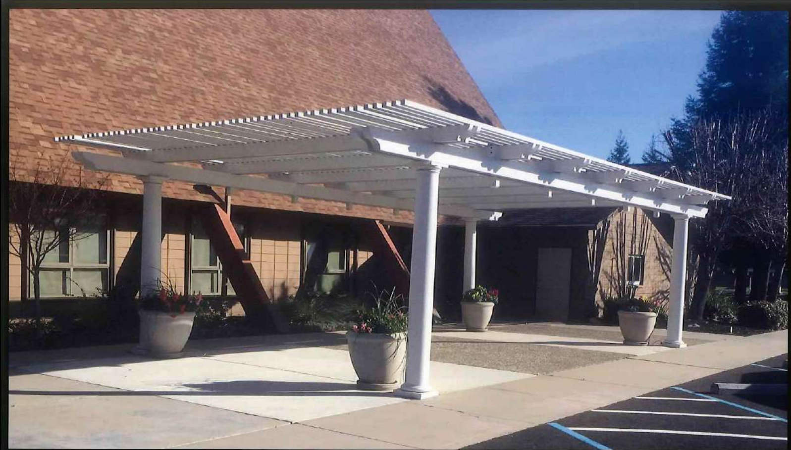
Ultra Lattice 2x2 lattice cover with double 2x6 rafters, double 3x8 beams, and 10" round columns
